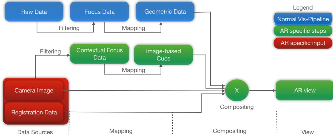
**Fig. 7:** AR visualization pipeline for extracting image-based physical cues. (Data sources) Important elements from the camera are extracted and (Mapping) mapped to an importance map that represents the physical cues. (Compositing) These cues are then combined with the camera image (for video see-through) and virtual geometries to create the final AR view.
