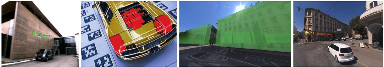
**Fig. 9:** Examples for using model-based physical cues. Left) Using aerial 3D reconstruction data for occlusion culling (Zollmann et al. [69]). Middle Left) A ghostings based on edges extracted from a registered 3D CAD model (Kalkofen et al. [105] ©[2009] IEEE). Middle Right) GIS data used for occlusion culling. Right) GIS data applied for occlusion culling (Skinner et al. [70]).
