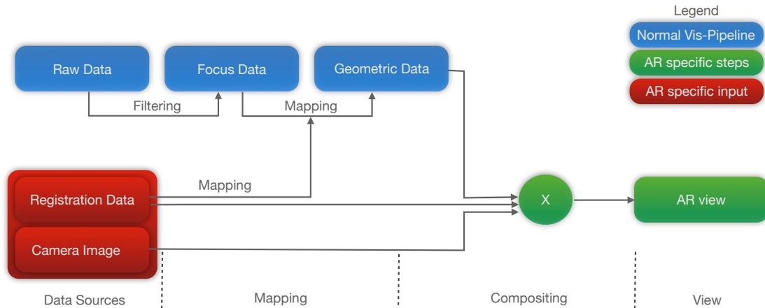
**Fig. 12:** Pipeline for mapping distance to appearance. The camera image is only needed for video see-through displays or when extracting other image features.
