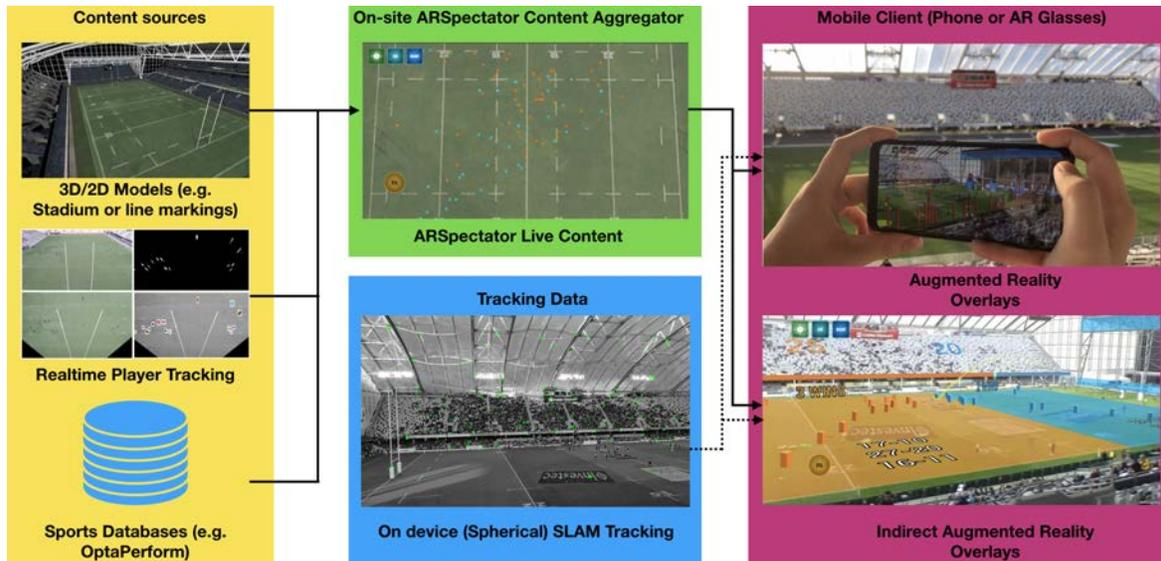
**Figure 2: ARSpectator overview. ARSpectator integrates sport-related data from different sources that are visualised via a direct AR or indirect AR interface.**
