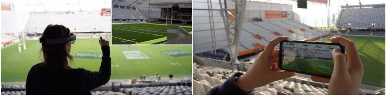
**Figure 1:** ARSpectator using the HoloLens and a mobile phone. Left) 3D structures of the stadium and line markings are overlaid using the AR interface on a HoloLens. Right) Sport related information is overlaid using ARSpectator on a mobile phone.
