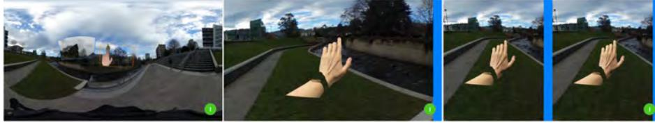
Figure 3.2: The possible ways to view the shared environment. (Left): An equirectangular projection of the entire panoramic space. (Centre): A first-person view of the environment based on the orientation of the user’s device. (Right): A pseudo-stereoscopic projection for viewing in a mobile HMD.
