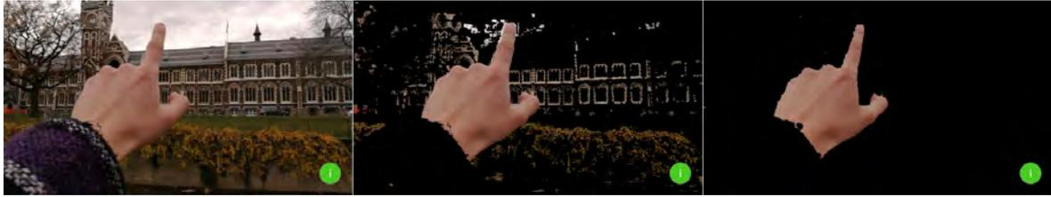
Figure 3.8: An example of the real-time skin segmentation the application can achieve. (Left): The original image. (Centre): The same image after colour-based segmentation. (Right): The image after distance-based thresholding on the segmentation mask.
