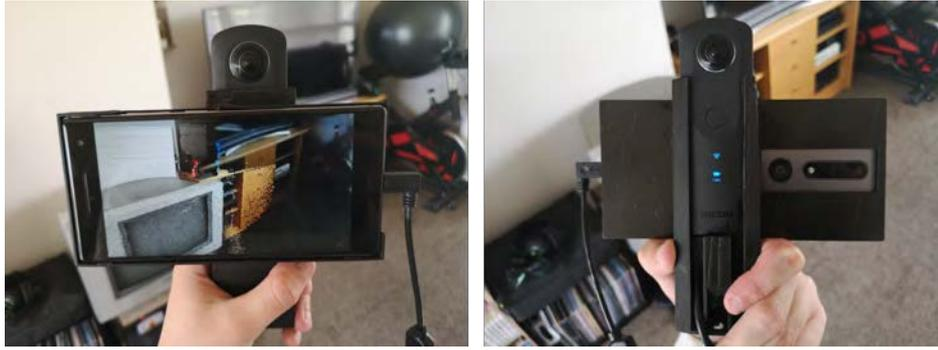
Figure 5.4: The hardware required for Mobileportation. The Lenovo Phab 2 Pro handles all tracking, rendering, reconstruction, and other computation, while the Ricoh Theta S provides 360° video capture and is connected to the phone via USB. The devices are combined using a purpose-built 3D-printed mount.
