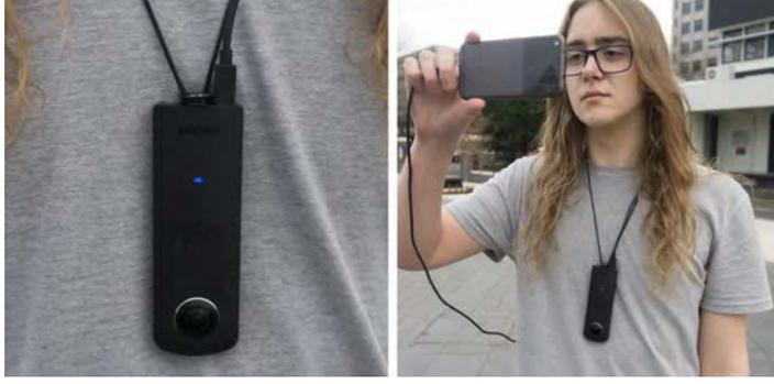
Figure 3.11: The Ricoh Theta S, a camera used for 360° image capture in Live Panoramic Video Calling. (Left): A close-up of the Theta being worn around the user’s neck. (Right): The Theta connected to a mobile phone via a USB cable.
