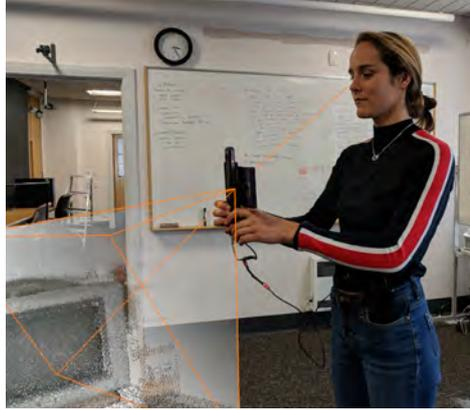
Figure 5.7: An example of how the user’s gaze direction could be used to affect their view of the environment. The angle between their face and the display is calculated and used to offset the angle of the render camera, allowing the display to be used as a “smart window” into the environment. Their gaze frustum is also offset by this same angle, allowing more precise indication of where they are currently looking.
