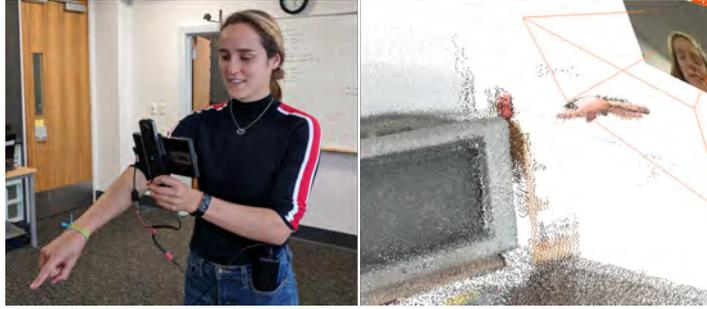
Figure 5.8: A user performing a pointing gesture within 3D space. Their hand is found within the latest point cloud capture using colour thresholding and only rendered temporarily so that gestures can be used without affecting environmental reconstruction.
