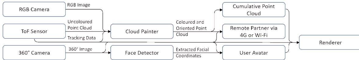
Figure 5.3: An overview of how data flows through the system’s various modules to give the overall experience. The data here moves from left to right, so all is captured by the RGB, ToF or 360° camera and passed through several modules before being rendered or sent to the remote peer.
