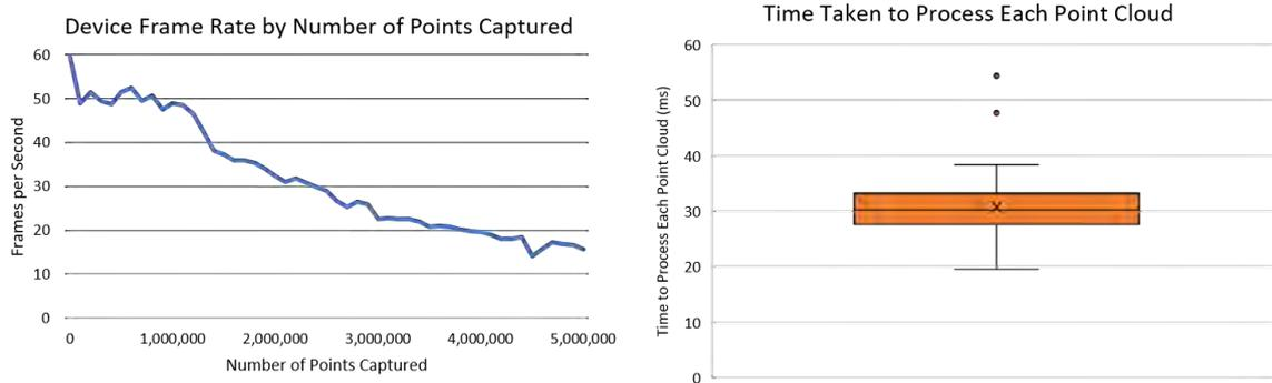
Figure 6.1: (Left): The application frame rate as a function of the number of points captured. More points result in a linear decrease in performance, though it remains interactive for all but the largest of captures. (Right): The time required to process each point cloud once it is captured. This averages 30ms in almost all cases, suggesting that 30fps capture would be possible with a more capable ToF sensor.
