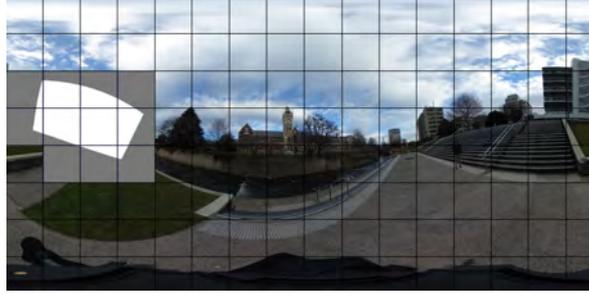
Figure 3.9: An illustration of how culling quads are overlaid on the panorama framebuffer to prevent the projection shader executing for every fragment. Here the white area shows the projection area and the grey squares show the quads that will have the shader executed on them. The coloured regions will not have the projection performed on them at all, drastically reducing computation time.
