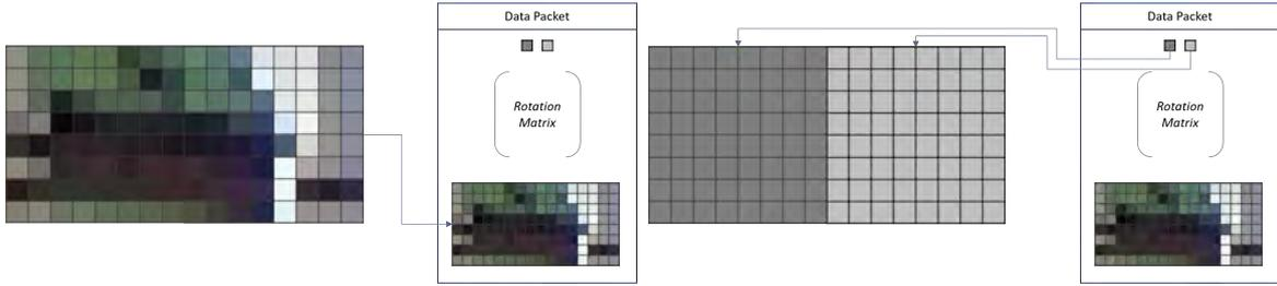
Figure 3.5: How the data packet’s identification is embedded in its corresponding image. (Left): Two 8x8 regions of pixels in the top-left corner of the image are removed and stored in the orientation packet. (Right): These pixels are replaced with the packet’s two-byte id tag. When received, this process allows these disparate packets to be synchronised and combined.
