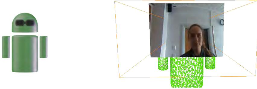
Figure 5.6: (Left): The model used to show each user’s position and orientation within the virtual space. It is first converted to a point cloud through offline subsampling to maintain visual coherence with the rest of the environment. (Right): The model once rendered into the environment. The user’s face is captured and overlaid to allow face-to-face communication, and a frustum is shown to indicate their gaze direction.
