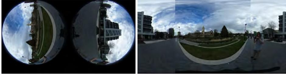
Figure 3.12: An example of the 360° images obtained by the Ricoh Theta S. (Left): The dual-fisheye format natively captured by the camera. (Right): The same image after being projected into the equirectangular panorama.
