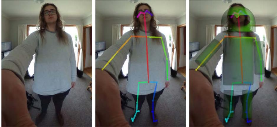
Figure 5.9: An example of how the user’s body can be tracked within the 360° video captured by the Ricoh Theta. (Left): The user as seen by the 360° camera. (Center): The user’s skeleton detected within this image using OpenPose. (Right): The position of the user’s limbs are used to manipulate their 3D avatar, allowing their actions to be properly displayed within the environment.
