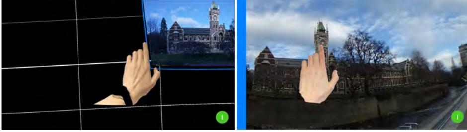
Figure 3.7: The indicator used to show each user’s current field of view. (Left): When the two users’ views overlap, a coloured box is drawn around the partner’s FoV to show where they are currently looking. (Right): When the two users’ views do not overlap, one edge of the screen will be coloured to show which direction the user needs to turn in order to see their partner’s view direction.
