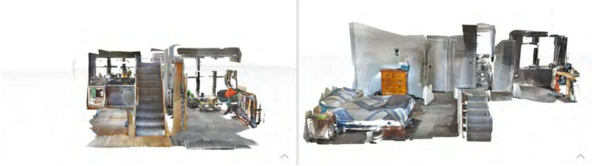
Figure 5.5: An example of a two-storied building that was reconstructed in real time using Mobileportation. Each floor is constructed separately for the sake of clarity, but the application is capable of producing this entire point cloud in one session, which would be difficult with traditional desktop systems tethered by cables and tracking spaces.
