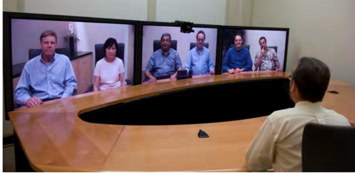
Figure 1.1: A Cisco Telepresence System<sup>1</sup>, currently seen as the state-of-the-art in enterprise telepresence solutions. While one could fool themselves that their conversational partner really is on the other side of the desk, this requires an entire room to be set aside for a very specific type of conversation that provides no meaningful interaction methods between users.
