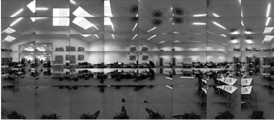
Figure 3.10: A pre-captured panorama after being split and unprojected into multiple segments to give undistorted views of each area within the space. These segments are stored along with the orientation with which they were obtained and their set of feature descriptors so that new frames can be positioned relative to them.
