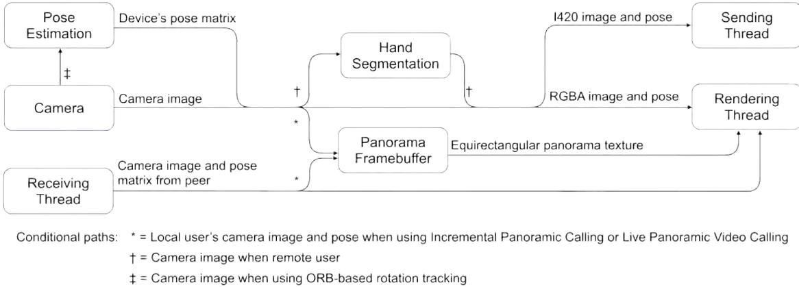
Figure 3.4: The low-level subsystems shared by each mode and the interactions between them. Paths marked \*, † or ‡ are only conditionally followed.
