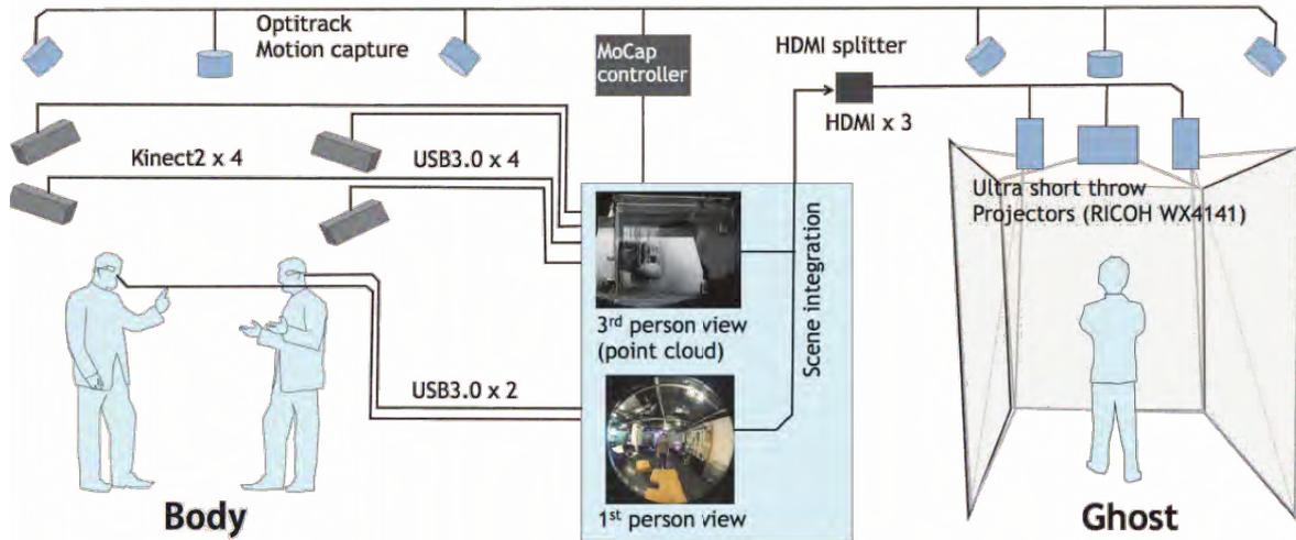
Figure 2.7: An illustration of Jackin Space (Komiya et al., 2017), which serves as a typical example of systems which use outside-in camera placement to reconstruct the shared environment.
