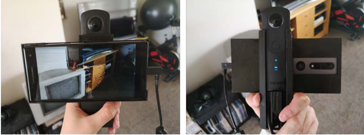
Fig. 3. The hardware used in our research. The Lenovo Phab 2 Pro is used for reconstructing and viewing the environment, while the Ricoh Theta S is used for capturing users' faces and live 360° video for egocentric viewing. The two devices are connected via USB and combined using a custom-built 3D-printed mount.
