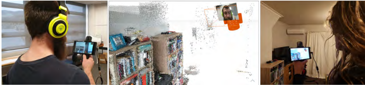
Fig. 1. Two users at different locations communicate within a shared environment constructed using consumer-grade mobile phones with an integrated RGBD sensor and external 360° camera. Here, the local user (right) shares his environment with the remote user (left). Both “meet” in an incrementally constructed shared virtual space (centre) where they can freely move between ego- and exocentric viewing positions. This reconstruction can be created and transmitted in real time over a standard cellular network, and each user’s position within it is shown as an avatar to allow for nomadic face-to-face communication.
