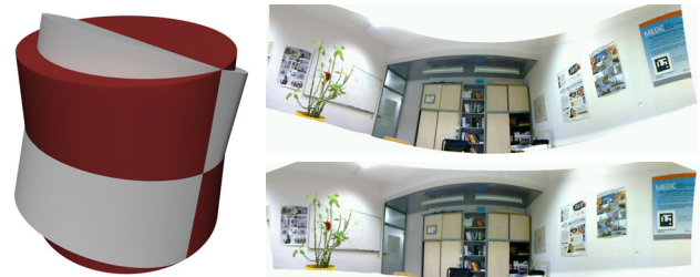
Figure 6. Left: Mapping from the reference cylinder (red) onto another cylinder (gray), tilted 20^\circ . Top-right: Effect of a pure horizontal camera movement after a wrongly initialized pitch angle. Bottom-right: The same map fixed using reprojection.
