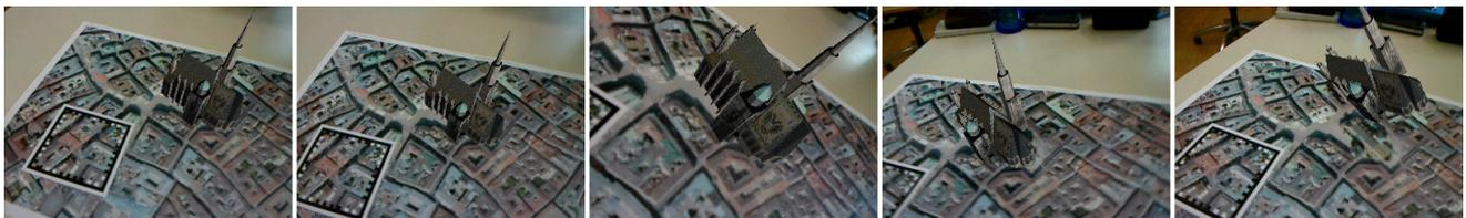
Figure 5: Incremental tracking over 400 frames ( $\sim 20$  seconds): 1<sup>st</sup> image (frame 17): pose estimated from marker, 2<sup>nd</sup> image (frame 53): incremental tracking takes over, 3<sup>rd</sup> image (frame 86): tracking still accurate, 4<sup>th</sup> image (frame 164): drift becomes obvious, 5<sup>th</sup> image (frame 381): tracking is completely off.
