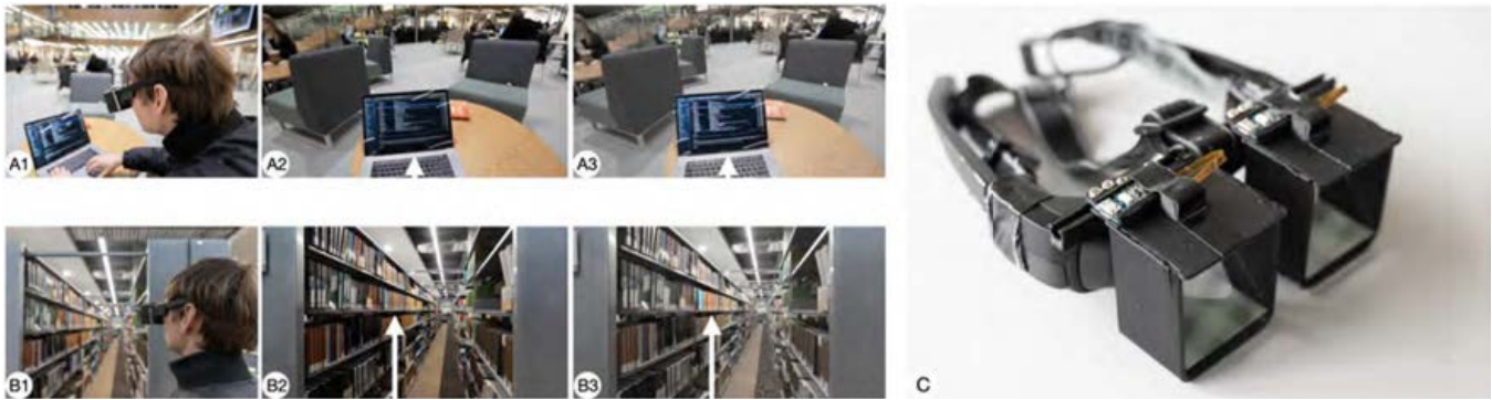
Figure 12: Two conceptual scenarios showing how the concept could be used for focusing on a main task (A) or finding objects (B). Our approach captures the real-world (A2 and B2) and modulates the saliency (A3 and B3) to guide the user’s gaze to modulated scene elements (here simulated output of the computer and books on the shelf subtly modulated with our algorithm, as intended for an unobtrusive guide). The white arrow pointing out the emphasised area is for illustration only. (C) Working mobile prototype combining a Lumus DK52 with integrated scene cameras for saliency modulation.
