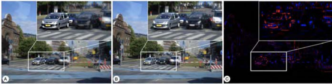
Figure 2: Differences in saliency modulation methods not considering additive only properties of OSTHMDs exemplified by our implementation of the algorithm by Mendez et al. [38] (insets for details): (A) Full colour control allows increasing the saliency of some image elements (e.g., silver car) while decreasing the saliency of other elements (e.g., black car). (B) Modulation using only the additive components fails to demonstrate the full saliency modulation. (C) Visualisation of required additive (red) and subtractive (blue) modulation necessary to highlight the silver car showing the majority of image areas are modulated by subtractions that are not possible in OSTHMDs.
