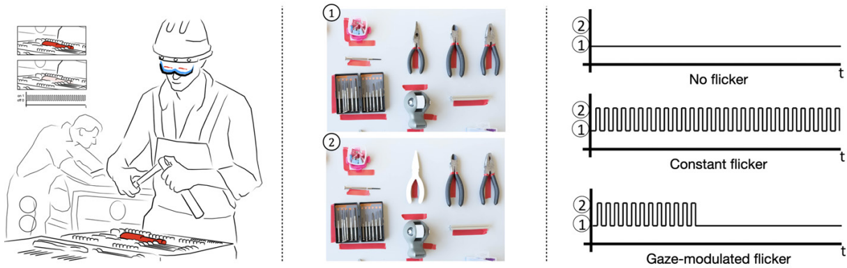
Figure 8: Conceptual overview on the study. (Left) Real-world visual guidance to emphasise tools or item in order picking tasks served as general inspiration for the task. (Middle) Flicker guidance is achieved by a rapid adjustment of brightness creating two alternating views when seen via the AR glasses (Right) Illustration of the three conditions with either no flicker, a constant flicker created by alternating between view 1 and 2, or a gaze-modulated flicker that ceases to flicker once gazed at.
