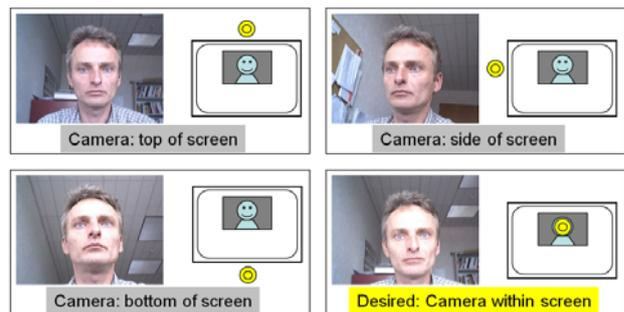
**Figure 1. Eye-to-eye contact: separation of camera and screen.**
