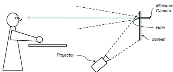
**Figure 2. Schematic of hole in screen approach**
