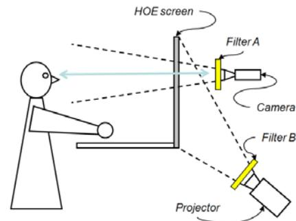
**Figure 7. Schematic of “i2i” (HOE and filters) approach**
