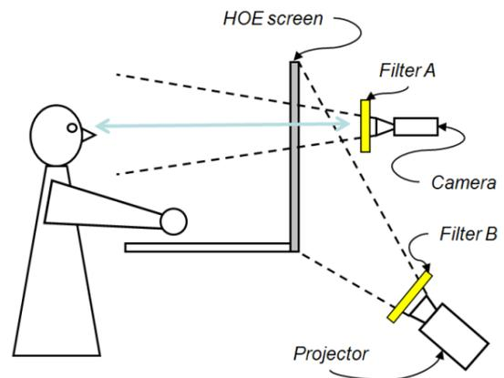
**Figure 2. Schematic of “i2i” approach. A Holographic Optical Element (HOE) is used to separate the camera view from the projected video conferencing image. Additional polarization filters are added in the light path.**
