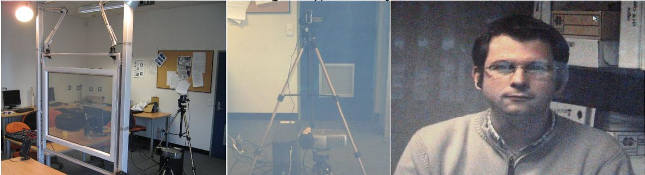
Figure 1: i2i system setup (left), see-through view shows the videoconferencing camera when no image is projected (centre), video conferencing result of our system showing eye-to-eye-contact (right).
