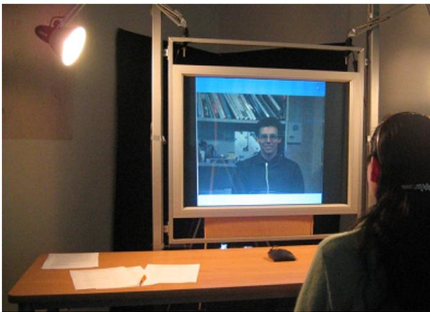
**Figure 3. The camera behind the HOE can't be seen by the users and only the image of the conferencing partner is visible providing eye-to-eye contact.**
