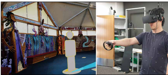
Figure 4. Left: Inside view including teleportation mechanism. Right: user wearing head-mounted display while exploring the virtual wharerau.
