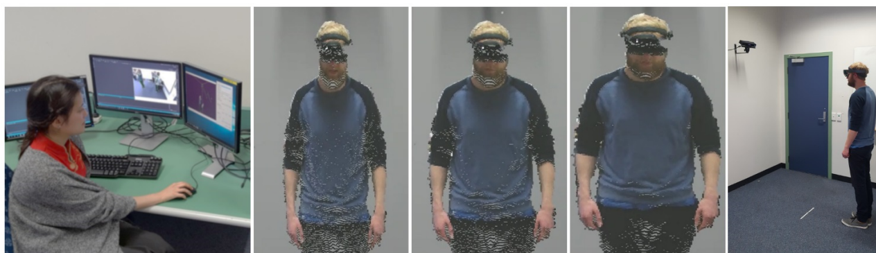
Figure 1: left—operator controlling 3D point cloud body size; center—three different body sizes; right—participant wearing the HoloLens in front of the Kinect capture sensor
