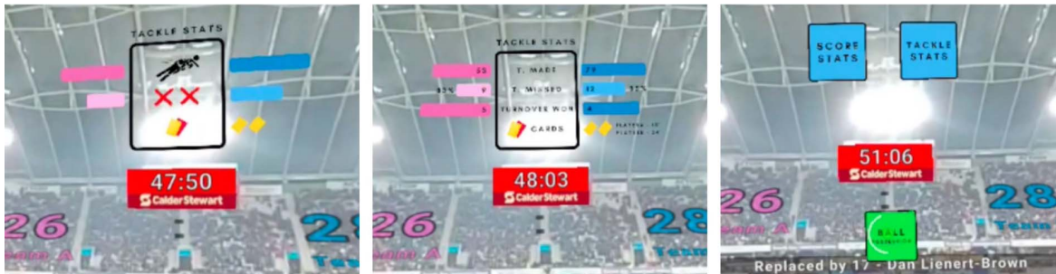
Figure 1: Our level of detail (LOD) implementation and context-aware adaptive AR interface for sports spectating: Left) A LOD-1 rugby tackle stats visualization which displays minimal information. Middle) A LOD-3 rugby tackle stats visualization with the maximum information shown if the user wants more details. Right) Part of the adaptive interface where users rely fully on context and head movement to interact. Shown is the LOD-0 icons for user to select.
