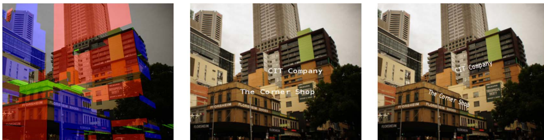
Fig. 13. Example of applying geometric constraints determined in real time from a single image. (Left) The computed surfaces and their orientation within the image. (Middle) The labels placed at their original position. (Right) Applying a layout algorithm based on geometric constraints such as the surface map and the edge map allows to automatically align the labels with their underlying geometry depicted in the current camera image.
