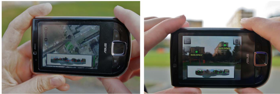
Fig. 5. Overview of the prototype demonstrating precisely anchored textual annotations in AR. (Left) Two-dimensional map overview showing spots with attached annotations. (Right) AR interface showing nearby textual annotations that are precisely matched against a panorama built in a background process.
