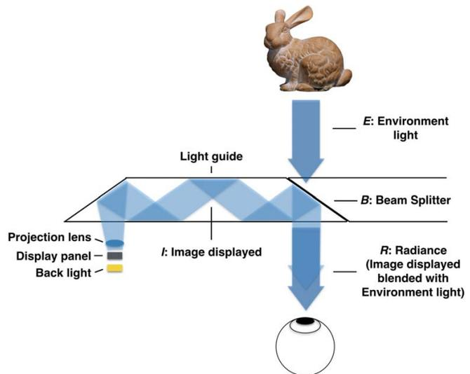
Fig. 2. Illustration of the basic functionality of a Optical see-through Head-Mounted Display.
