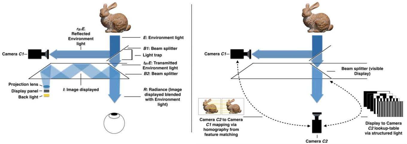
Fig. 3. Schematic overview over our OHMD prototype. (Left) The addition of a beam-splitter allows to partially reflect the incoming environment light towards the camera  $C1$ . (Right) To allow for a pixel-precise mapping between the camera  $C2$  (representing the users eye for our tests) and camera  $C1$  we apply a camera display calibration using structured light and a camera-to-camera mapping using a homography.
