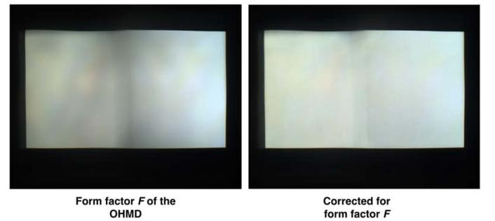
Fig. 5. Example of measuring and correcting the form factor  $F$  describing the light falloff in the OHMD caused by optical imperfections in the display: (Left) Displaying a white image in front of a uniform black background gives the form factor  $Fr_{B2}$ . (Right) Compensating only for  $Fr_{B2}$  result in a more uniform image (here demonstrated again with a white image). Both images are not cropped and recorded through the eye camera  $C2$ .
