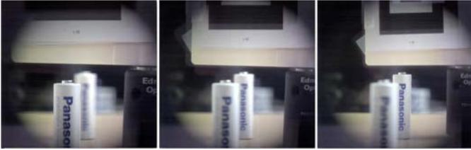
Fig. 11. Continuous Single Focus controlled by placement of a fiducial marker. Focus is set to distance given by marker position (left) Focus is on object in front. (center) Focus is set to be between front and back object. (right) Focus is on back object.
