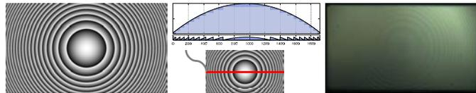
Fig. 2. A PSLM can display a computational lens. (left) An input spherical phase pattern. (middle) The intersection of the pattern. The pattern is a Fresnel lens of a convex lens. (right) An actual lens image captured while focusing at the surface of the PSLM. The phase pattern behaves as if there is a thin lens layer on the PSLM.
