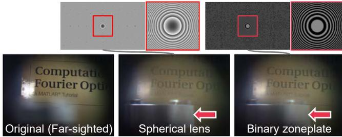
Fig. 9. Diffraction lens demonstration. A viewpoint camera focuses at a far object. We display a spherical lens phase pattern and a binary zone plate phase pattern of the same focal length separately. The resulting images in the bottom center and in the bottom right both focus on a near object. Note that the binary intensities of the zone plate image so that their retardation is a half of the base wavelength.
