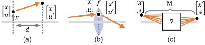
Fig. 4. Ray transfer matrix analysis. (a) A ray transfers space. (b) A ray transfers a thin lens. (c) Two points that are conjugate each other for a given ray transfer matrix.
