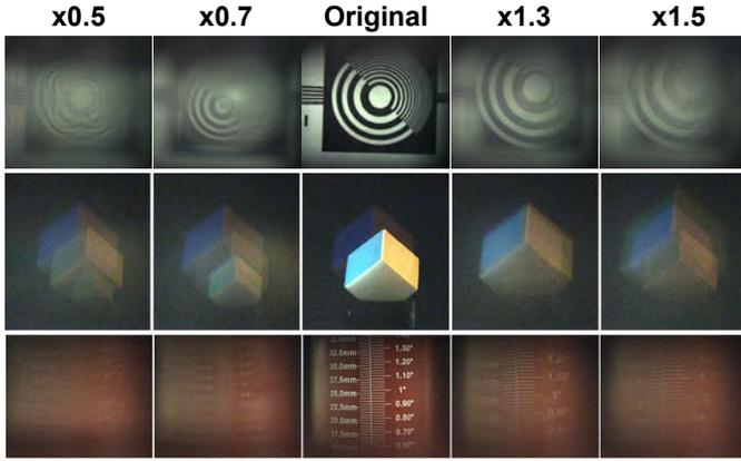
Fig. 14. The summary of the zoom control experiment with the dual-PSLM setup showing remaining artifacts which can be further reduced by increasing the view brightness. Three different backgrounds with four magnification rates are captured.
