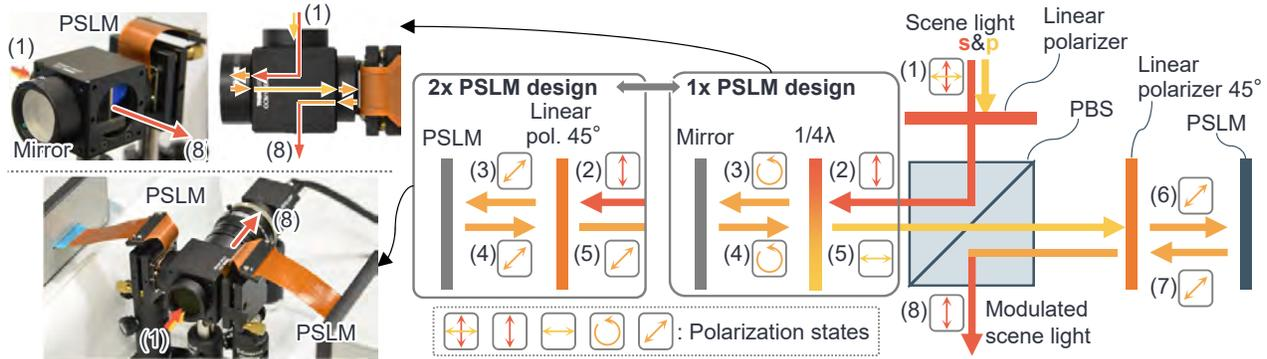
Fig. 7. Schematic diagrams of our optical designs and prototype systems. The right part illustrates how the system delivers the scene light from the world to the user's eye through PSLM(s) while avoiding the scene light directly reaching to the user's eye. See Sec. 4.1 for more details.
