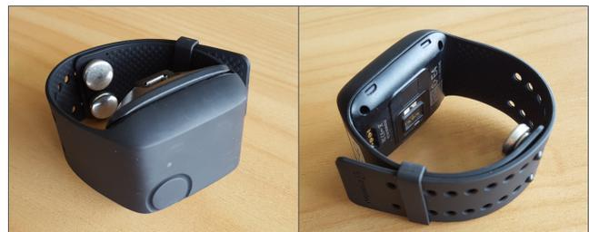
Figure 3: Empatica E4 wristband device for collecting physiological data used in our ERVE methodology. The exposed sensors can be seen in each view of the device.
