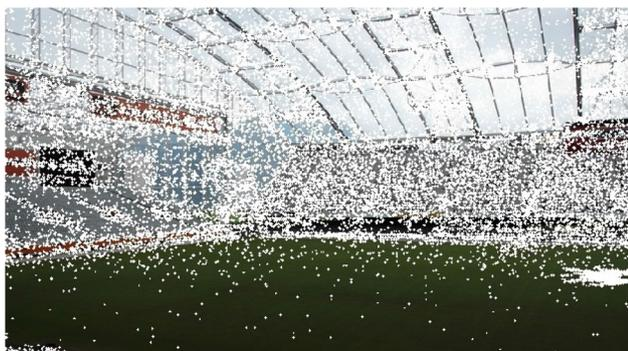
**Fig. 7** Example of accurate localization results from ESAC on the RS dataset. We render the sparse point cloud from COLMAP over the input images using the pose estimate. An accurate localization results in good alignment of the keypoints (white) with their corresponding structures in the image
