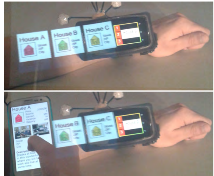
Fig. 6. In MultiFi [34] the appearance of user interface widgets can be adapted based on the characteristics of employed display devices, the presence or absence of individual displays and their spatial relationship. Here, a low fidelity card widgets seen through a low resolution, low contrast head-mounted display (top) turn into higher fidelity widgets once a smartphone is superimposed (bottom).
