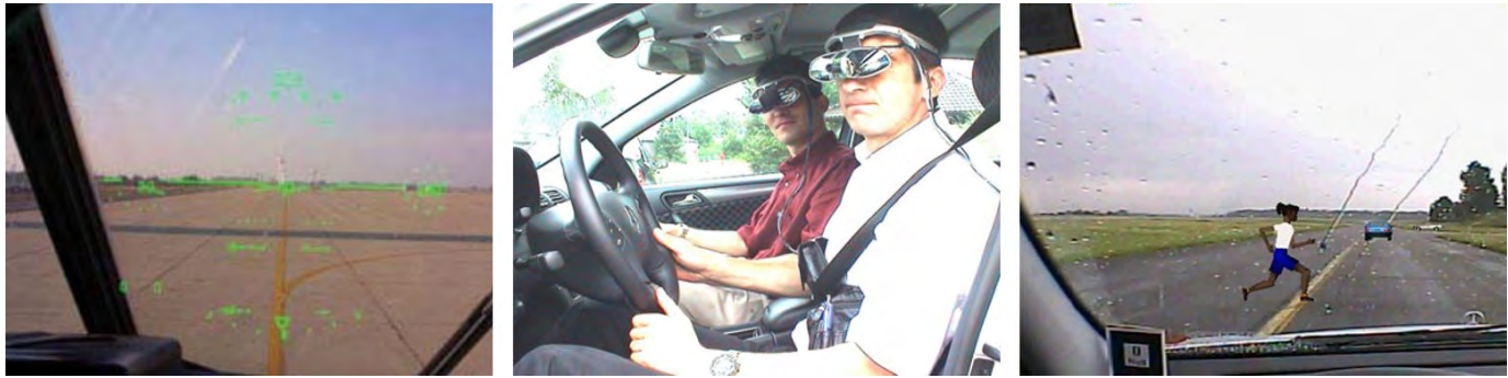
Fig. 2. Examples for context-aware information overlay applications (Left) A head-up display in the pilot's view in a fighter airplane [10], (Middle and Right) Driver and trainer in an AR-based driver training setup and a virtual car and child embedded into the driver's view [7].
