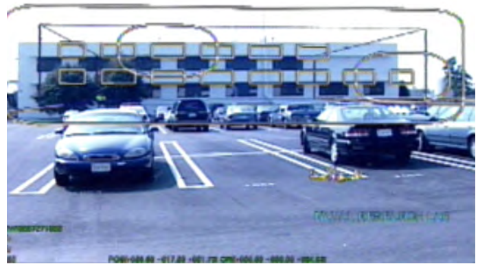
Fig. 7. Adapting to tracking error. A statistical determined average tracking error is used as adaption source to adapt the visual representation. The system highlights a physical building and two of its windows by outlining the area of the screen the objects could occupy (image by MacIntyre et al. [119]).
