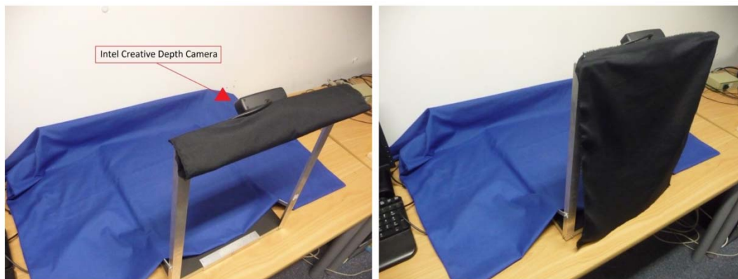
Figure 2. Metal Frame used to position the depth cam without curtain (left) and with the curtain to prevent the direct vision of the hand during use (right)
