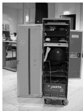
**Figure 6: Final AR system integrated into trolley**
