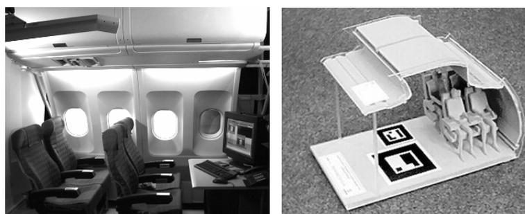
**Figure 5: a) Mockup of real-size cabin, b) Miniature cabin model**
